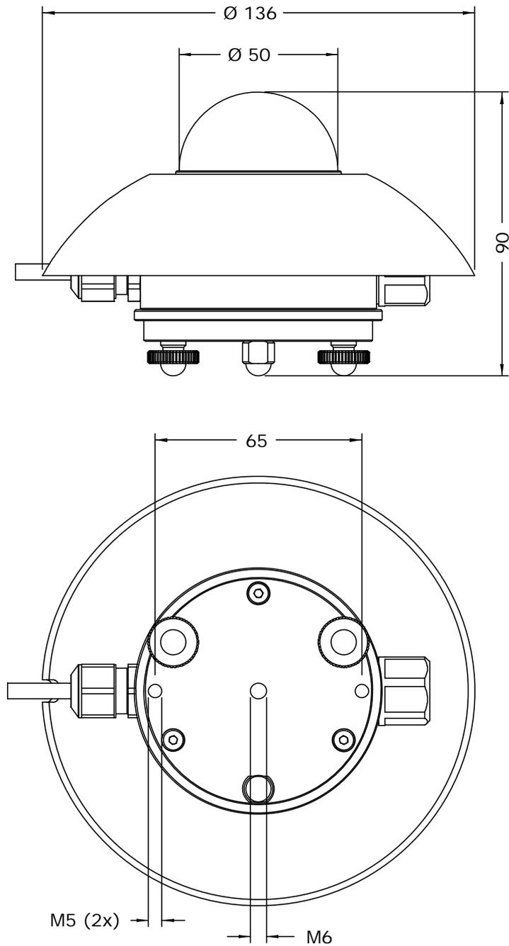
**Figure 3.2.1** Dimensions of SR12 in  $10^{-3}$  m.
