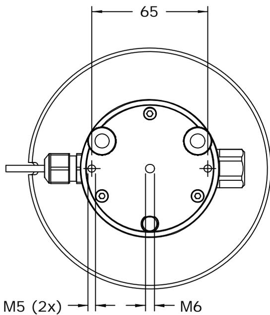
**Figure 8.2.2** Dimensions of SR12-TR in  $10^{-3} m$
