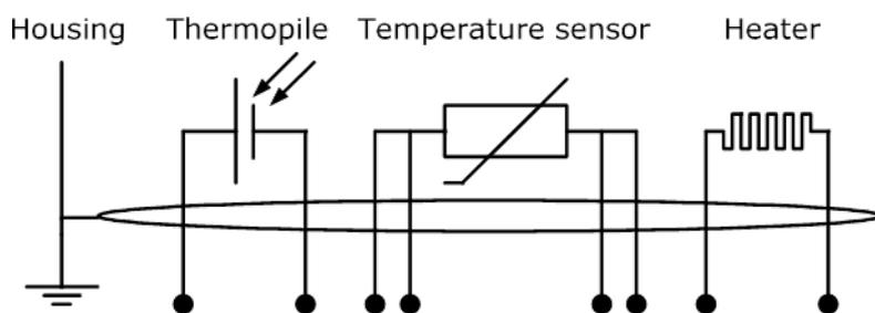
**Figure 5.3.1** Electrical diagram of SR12. The shield is connected to the sensor body.
