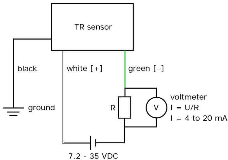
**Figure 8.3.3** Electrical diagram of the connection of SR12-TR to a typical voltmeter or datalogger with the capacity to measure voltage signals. Usually a 100  $\Omega$  shunt resistor ( $R$ ) is used to convert the current to a voltage. SR12-TR operates on a supply voltage of 7.2 to 35 VDC.
