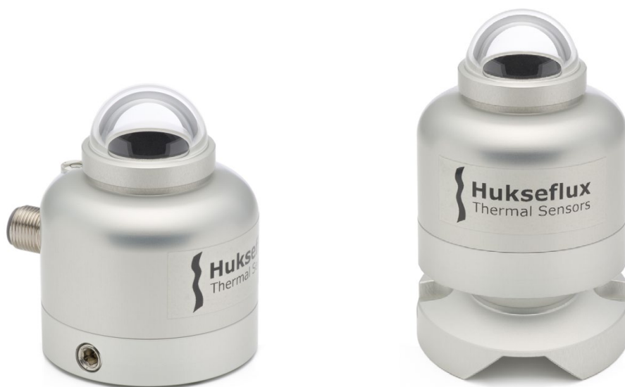
Figure 0.1 On the left SR05 digital second class pyranometer with bubble level and M12-A cable connector in its standard configuration (3 metre cable standard included); on the right SR05 with optional ball levelling, for easy mounting and levelling on (non-)horizontal surfaces (included mounting screws not displayed)
